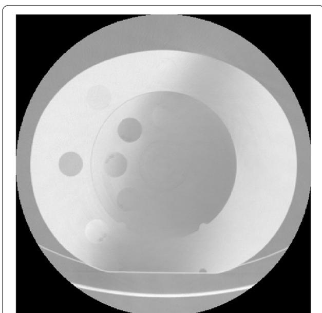
**Fig. 2** A DICOM image with a large artifact from the study’s phantom
