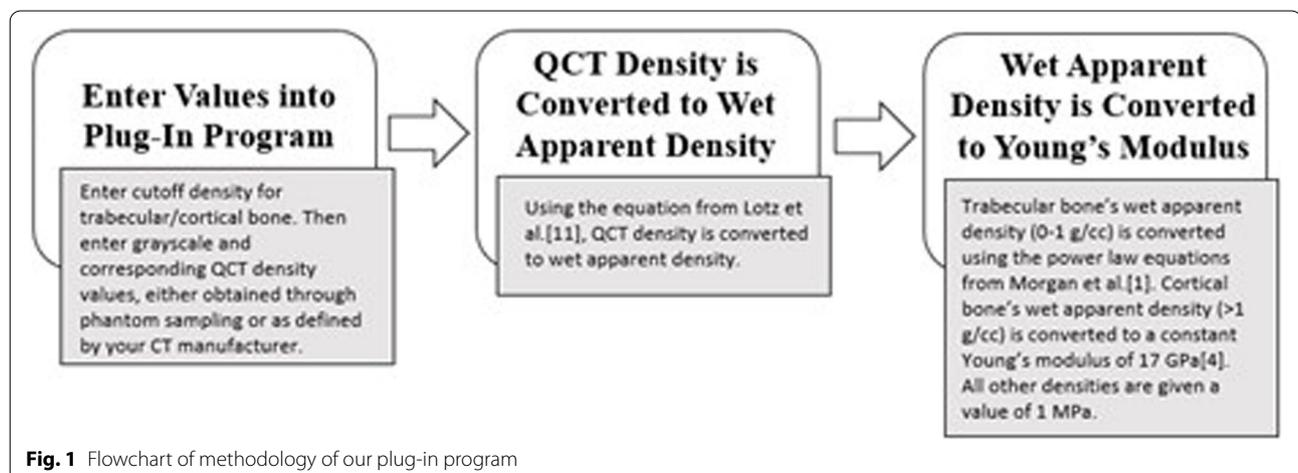
**Fig. 1** Flowchart of methodology of our plug-in program
