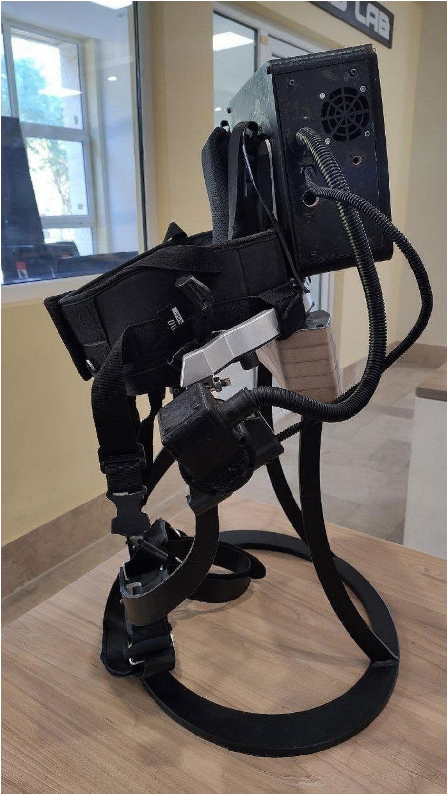
Fig. 1 Hip exoskeleton assistive (HEXA) robot
